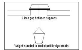
The bridge may be of any design but MUST conform to the specifications stated above. If the bridge does not meet the specifications, it will be disqualified from the competition. The toothpicks are to be the primary stress (load) carrying elements. The glue is to be used only to transfer stress (load) between toothpicks.
